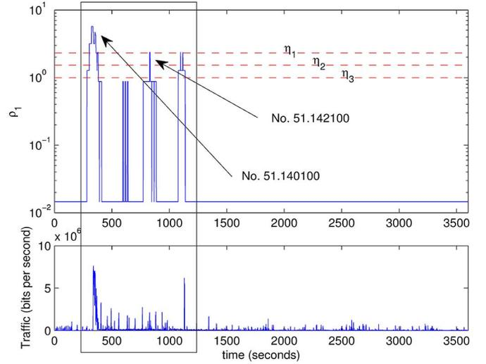
Fig. 8. Model-free method. (top) Value of  $I_1(p_{t,w})$ —Monday, fifth week (with attacks) between 2:00 pm–3:00 pm. (bottom) Outbound traffic—Monday, fifth week (with attacks) between 2:00 pm–3:00 pm. The rectangle identifies the time period there was an attack.
