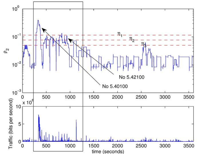
Fig. 9. Model-based method. (top) Value of  $I_2(q_{t,n})$ —Monday, fifth week (with attacks) between 2:00 pm–3:00 pm. (bottom) Outbound traffic—Monday, fifth week (with attacks) between 2:00 pm–3:00 pm. The rectangle identifies the time period there was an attack.
