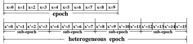
Fig. 4. A numerical example for a heterogeneous network with parameters  $m = 0.2$  and  $\alpha = 3$ , and  $p_{opt} = 0.1$ . We define  $x = r \bmod \frac{1}{p_{opt}}$ , and  $x' = r \bmod \frac{1}{p_{nrm}}$ , where  $r$  is the current round.
