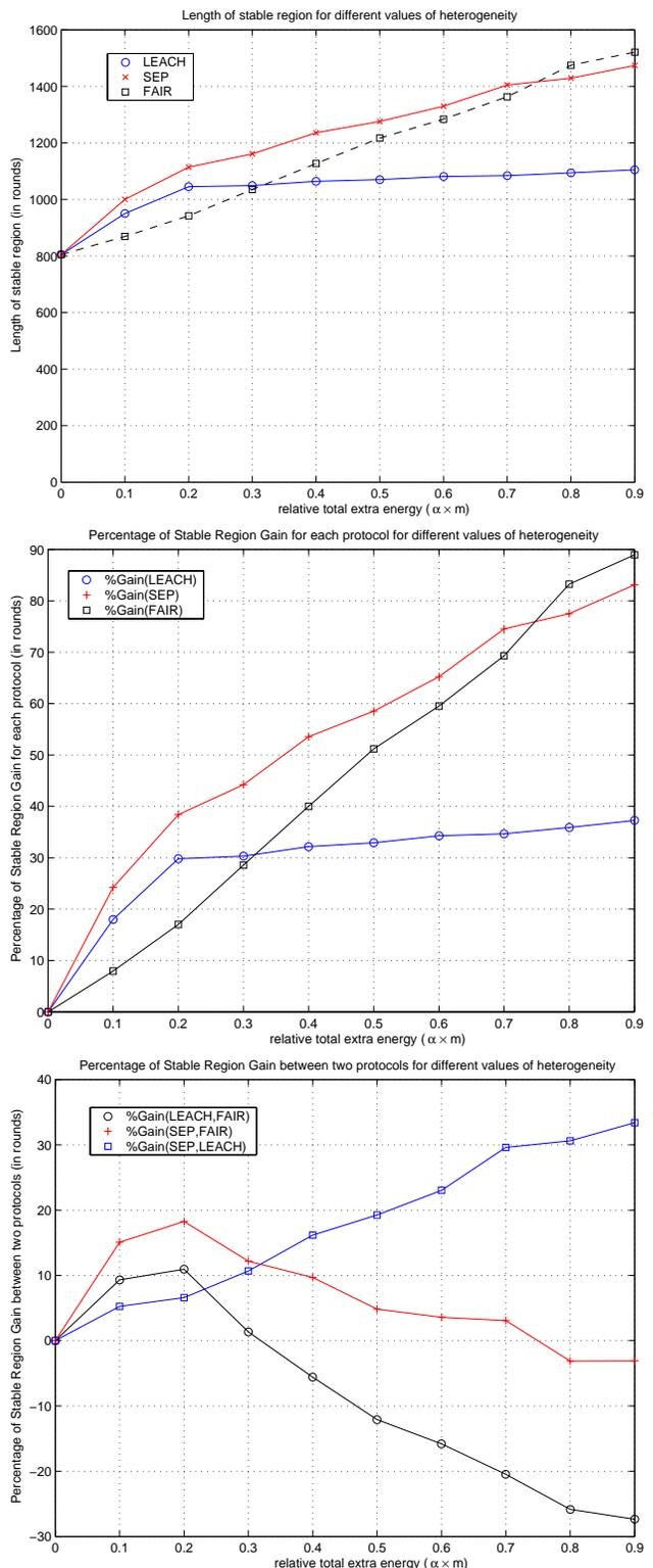
Fig. 9. Sensitivity of LEACH, SEP, and FAIR to degree of heterogeneity in small-scale networks.
