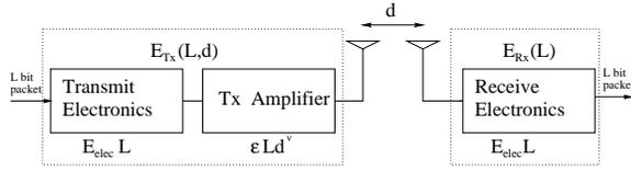
Fig. 1. Radio Energy Dissipation Model.
